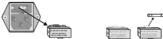
[ Replacing the Fuse ]
