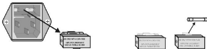
[ Replacing the Fuse ]
